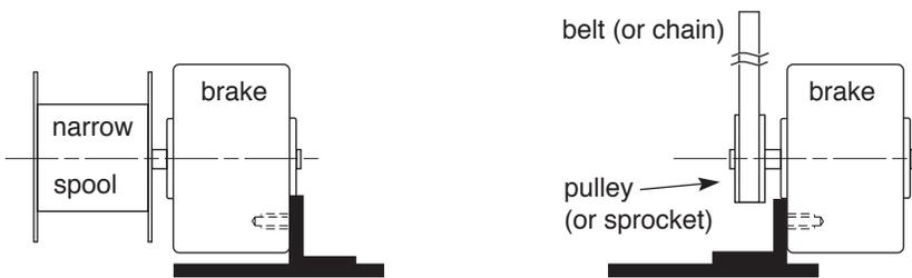
Belt, chain drive, or gears: The belt or chain flexes for misalignments. Gear play accommodates for misalignments. A bracket rigidly locates the brake.
