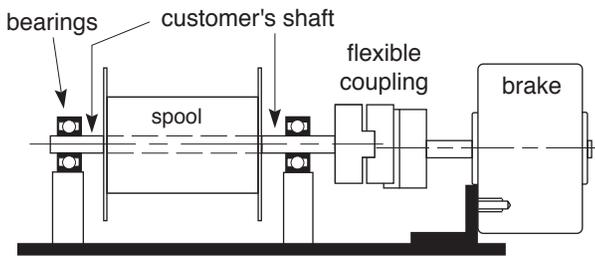
Both shafts fully supported by bearings - The brake shaft is supported by bearings. The customer's shaft (for the spool, or gearbox, motor, or any device) is also fully supported by bearings. Even with precise alignments, a flexible coupling is required. If a rigid coupling is used, the shafts are forced into alignment by bending the shafts, resulting in bearing overload, and premature failure.
