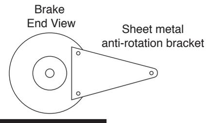
Floating solid-shaft brake - The customer's shaft for the spool (or other device) supports the rigid coupling, which supports the brake. The sheet metal anti-rotation bracket prevents the brake from rotating, yet flexes for misalignments. **Do not mount the brake housing rigidly.**
