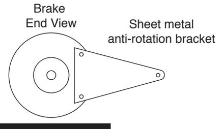
Floating hollow-shaft brake - The customer's shaft for the spool (or other device) supports the brake. The sheet metal anti-rotation link or bracket prevents the brake from rotating, yet flexes for misalignments.
