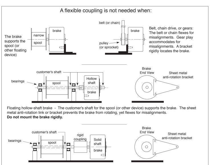
Floating solid-shaft brake - The customer's shaft for the spool (or other device) supports the rigid coupling, which supports the brake. The sheet metal anti-rotation bracket prevents the brake from rotating, yet flexes for misalignments. **Do not mount the brake housing rigidly.**
