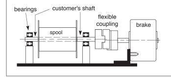
Both shafts fully supported by bearings - The brake shaft is supported by bearings. The customer's shaft (for the spool, or gearbox, motor, or any device) is also fully supported by bearings.
