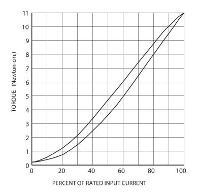
CHARACTERISTICS - With no electrical excitation, the shaft freely rotates. With electrical excitation, the shaft becomes coupled to the housing. Torque is proportional to input current (see torque graph), and independent of RPM. While the load torque is less than the output torque, the shaft won't rotate. When the load torque is increased, the brake will slip smoothly at the torque level set by the coil input current.
