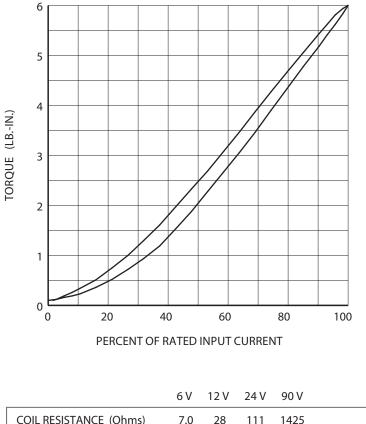
COIL RESISTANCE (Ohms) 7.0 28 111 1425 100% INPUT CURRENT (Amps) 0.77 0.39 0.19 0.067
