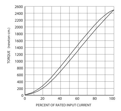
CHARACTERISTICS - With no electrical excitation, the shaft freely rotates. With electrical excitation, the shaft becomes coupled to the housing. Torque is proportional to input current (see torque graph), and independent of RPM. While the load torque is less than the output torque, the shaft won't rotate. When the load torque is increased, the brake will slip smoothly at the torque level set by the coil input current.
