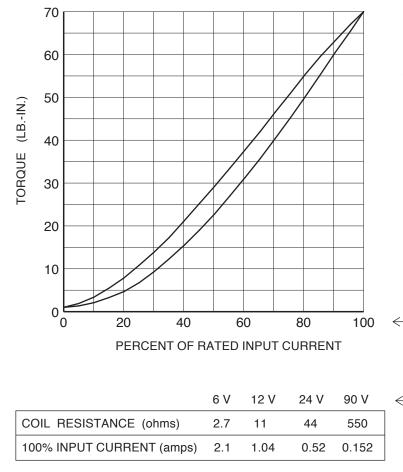
**CHARACTERISTICS** - With no electrical excitation, the input shaft & output shaft freely rotate. With electrical excitation, the input shaft becomes coupled to the output shaft. Torque is proportional to input current (see torque graph), and independent of slip RPM. While the load torque is less than the output torque, the clutch drives without slip. When the load torque is increased, the clutch will slip smoothly at the torque level set by the coil input current.
