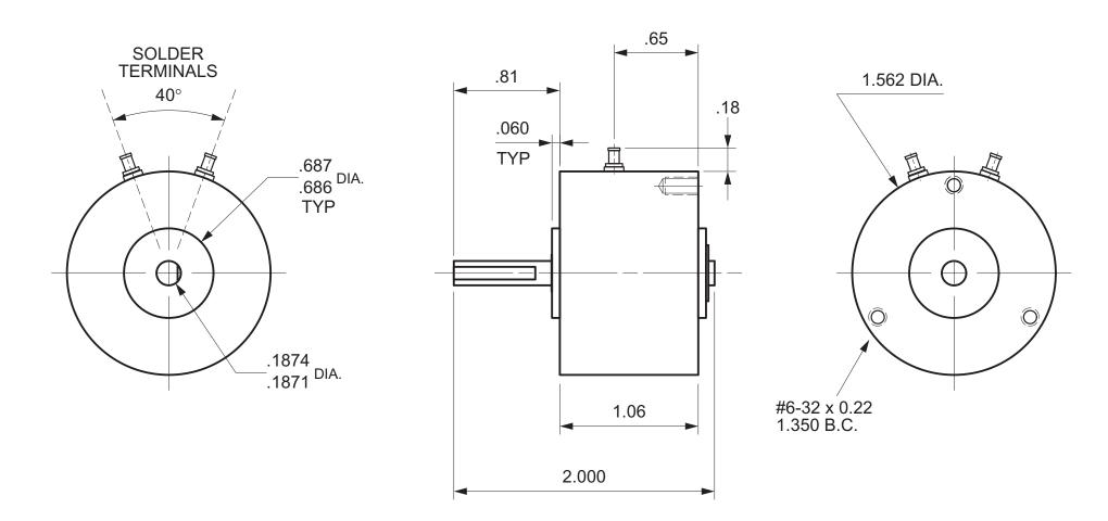
B1-1FR, Shaft out 1 side, (as shown)B1-1F, Shaft out 1 side, same side as mounting holesB1-2F, Shaft out 2 sides
