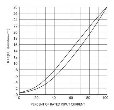
CHARACTERISTICS - With no electrical excitation, the shaft freely rotates. With electrical excitation, the shaft becomes coupled to the housing. Torque is proportional to input current (see torque graph), and independent of RPM. While the load torque is less than the output torque, the shaft won't rotate. When the load torque is increased, the brake will slip smoothly at the torque level set by the coil input current.
