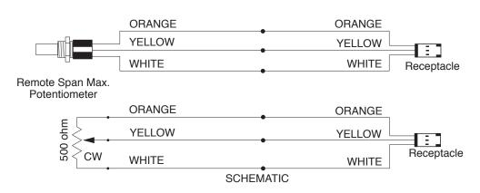
Connect the 3 contact receptacle, to 'D', (marked 'Remote') on power supply circuit board.
