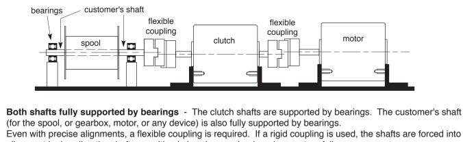
alignment by bending the shafts, resulting in bearing overload, and premature failure.
